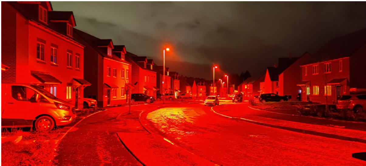
Photo 8: Red spectrum street luminaires deployed as lighting mitigation on a residential estate's spine road, at Lea Castle, Kidderminster. Image credit: Cody Levine.
